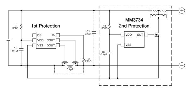
·R3 and C4 stabilize a supply voltage ripple. However, the detection voltage rises by the current of penetration in IC of the voltage detection when R3 is enlarged, and the value of R3 is adjusted to 1kohm or less. Moreover, adjust the value of C4 to 0.01 µF or more to do the stability operation, please.
