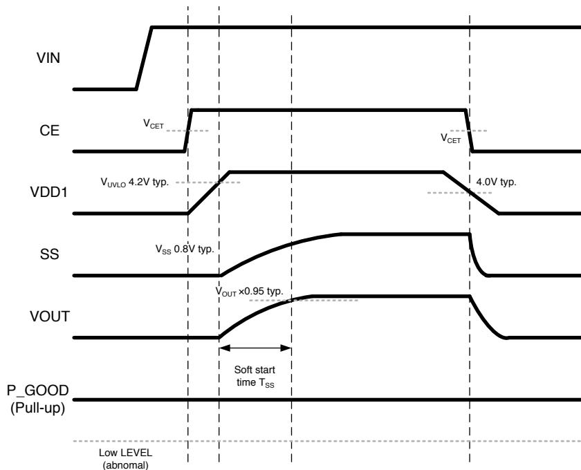
Start-up condition is  $V_{CE} > V_{CET}$  and  $V_{DD1} > V_{UVLO}$ .
