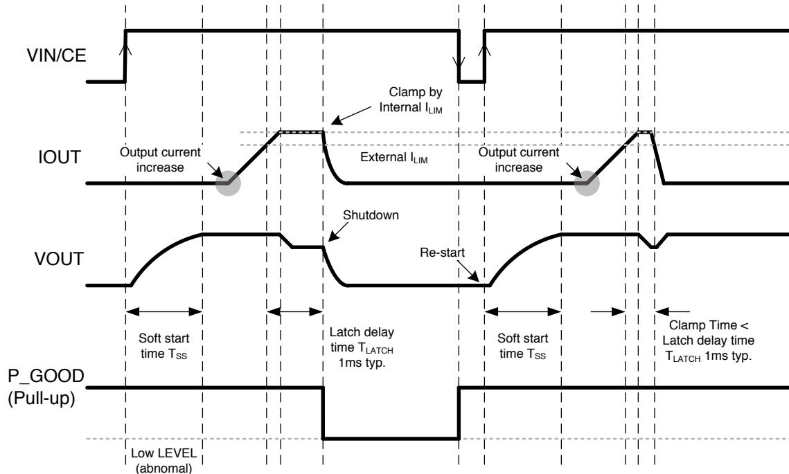
When Current limit are detected exceeding latch delay time  $T_{LATCH}$ , IC is shutdown, P\_GOOD is L-Output. The IC is re-start by turning on VIN/CE pin.
