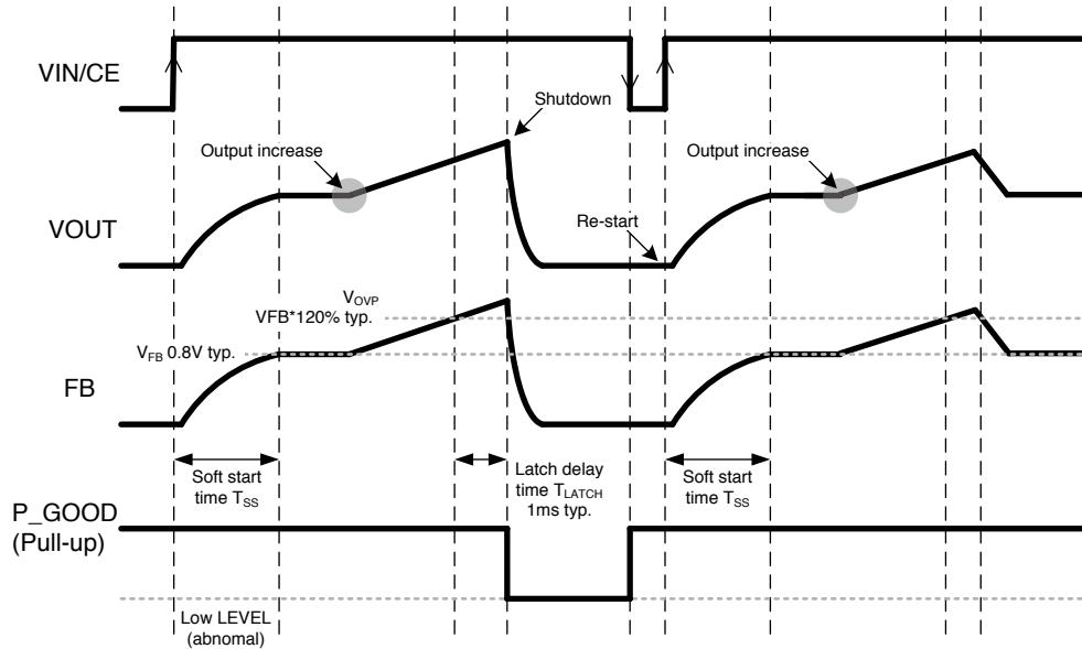
When OVP are detected exceeding latch delay time  $T_{LATCH}$ , IC is shutdown, P\_GOOD is L-Output.
