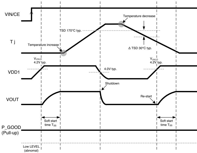
When the junction temperature ( $T_j$ ) rises above  $170^{\circ}\text{C}$ , VDD1 stops, and the IC shuts it down.
