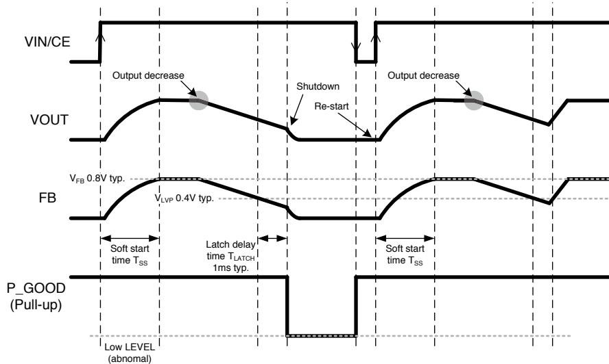
When LVP are detected exceeding latch delay time  $T_{LATCH}$ , IC is shutdown, P\_GOOD is L-Output.
