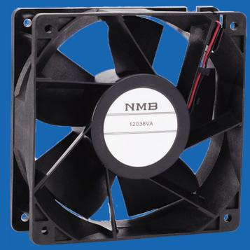
In addition to protection from external contaminants, NMB's IP69K fan are available with pulse-width modulation (PWM) speed control. Our customers can expect longer fan life with PWM speed control - the fan will spin faster only when required, thus reducing bearing load and wear. Power consumption will also be reduced because the fan will demand less power draw according to the duty cycle required.
