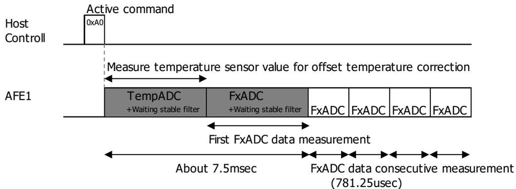
Fig. 11 Schematic of AD conversion start instruction
