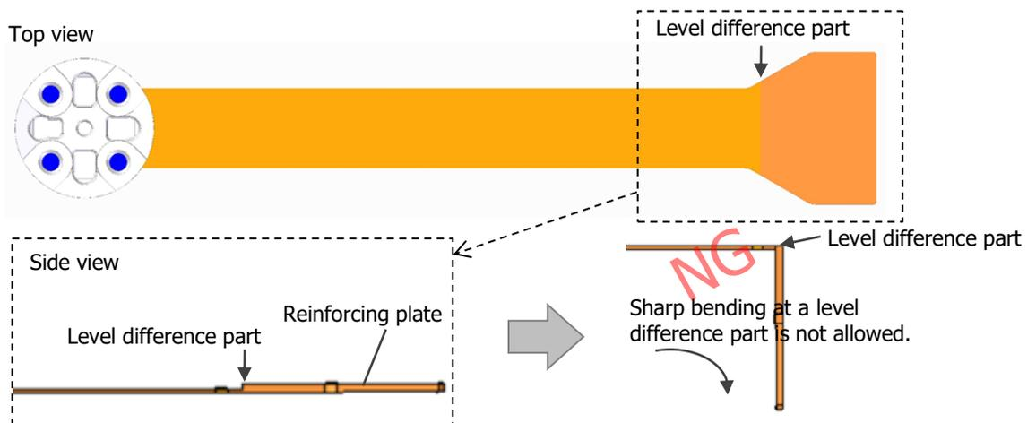
Fig. 38 Precaution for handling of sensor FPC - 2
