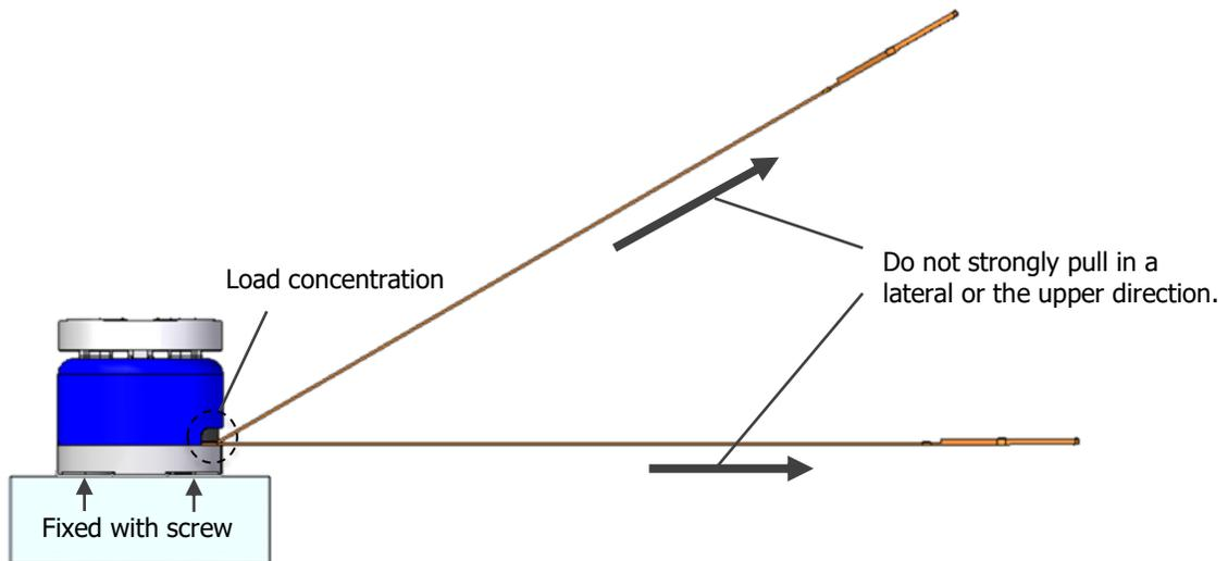
Fig. 37 Precaution for handling of sensor FPC - 1
