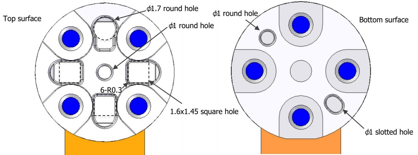
Fig. 34 Positioning holes
