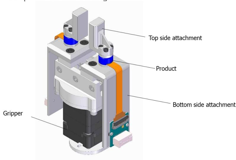
Fig. 28 Gripper-mounted image
