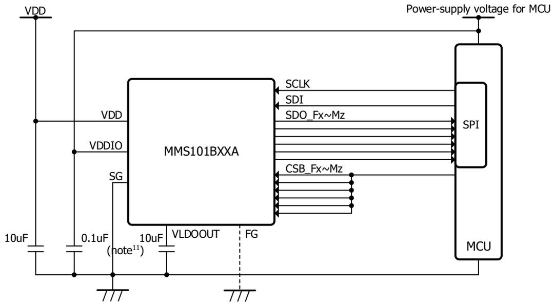
Fig. 24 Integrated CSB pin – Example application circuit
