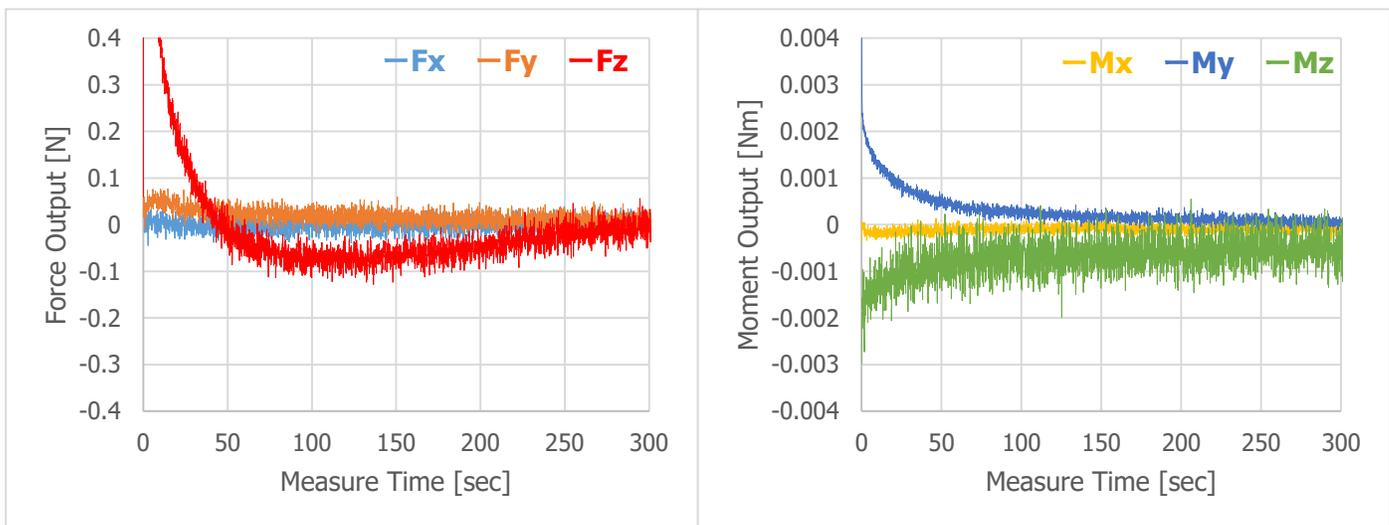
Fig. 12 Outputting data immediately after AD conversion starts
