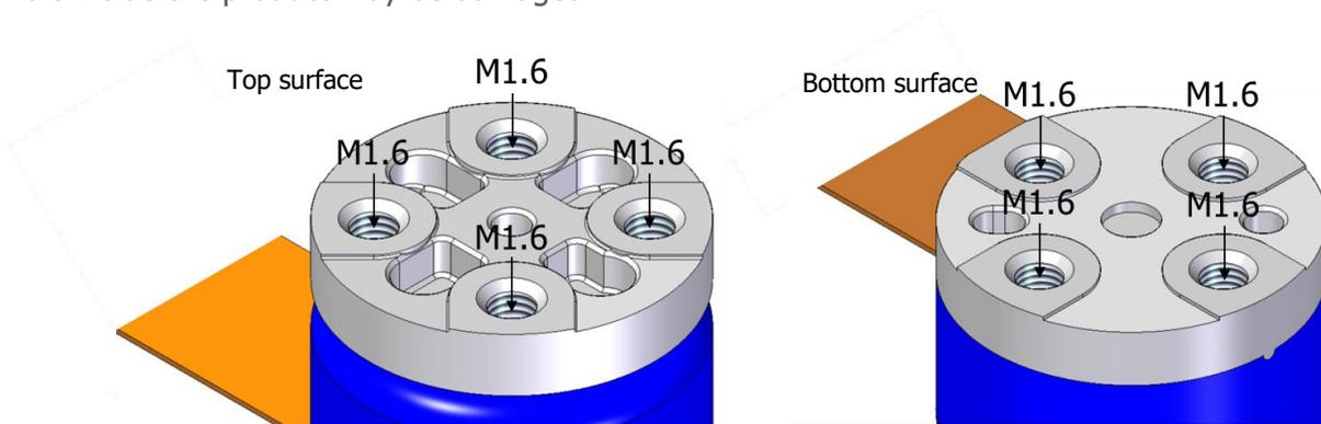
Fig. 32 Installation screw holeIn
