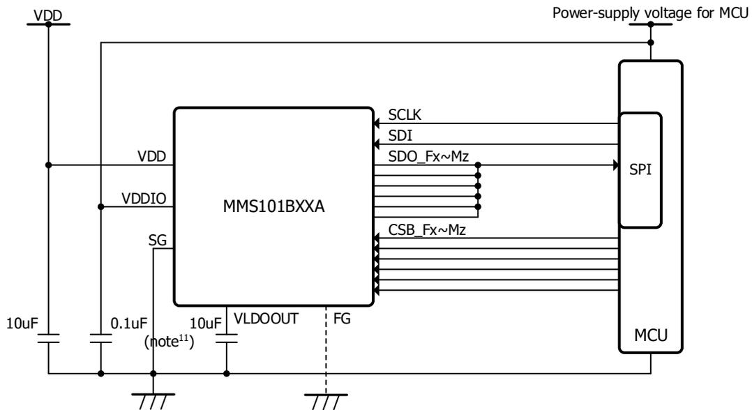
Fig. 25 Integrated SDO pin – Example application circuit
